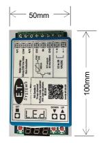
The **ET-RXCONDO-3** Universal Condominium Receiver has a digital display, any of the 999 users can programmed across all 3 channels and can be edited individually without effect to any other users already programmed into the memory.
