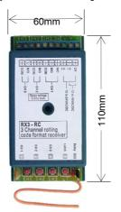
The **ET-RX3-RC** Universal Radio Receiver allows for Pulse, Latch or unique programmable up to 55 secs sustained/delay pulse output.
